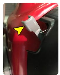
Always start the engine with the throttle moved UP to the idle position. (at the idle position the pump is not engaged)
