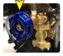
Once engine is started, adjust throttle and pressure to desired levels.
